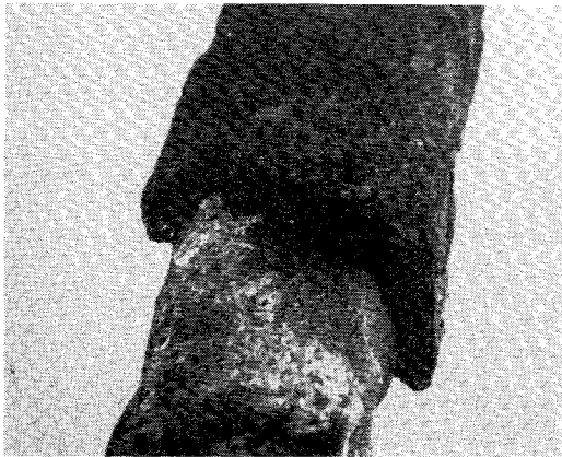
Figure 3 A length of cast iron where the fragile graphitised layer has partially exfoliated
