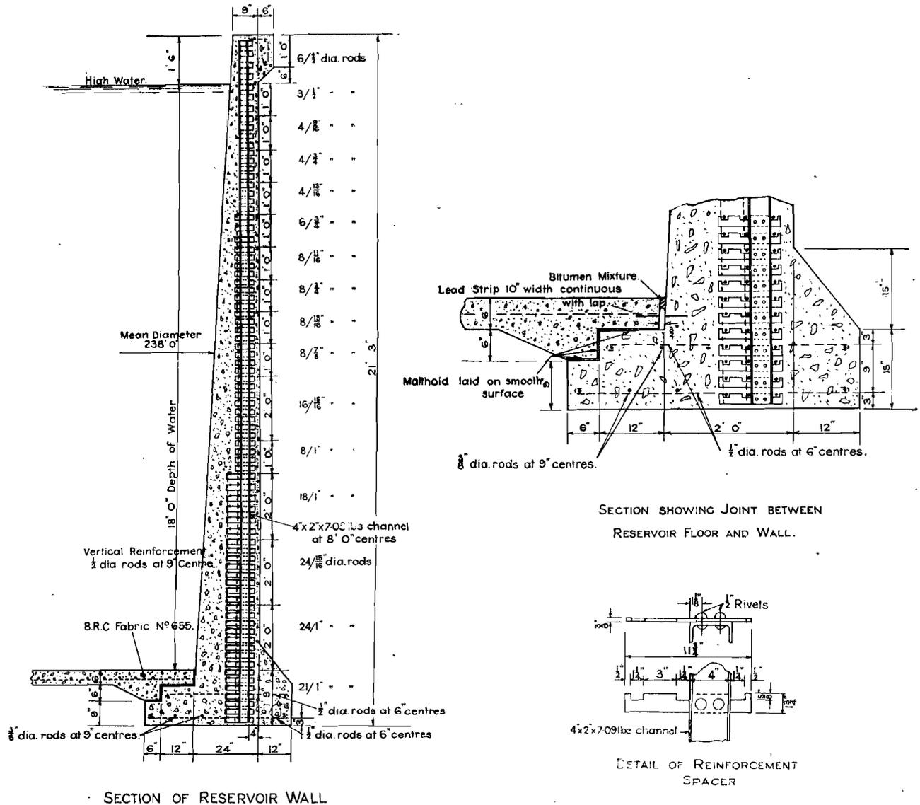
Fig. 3. Details of 5,000,000-gal. Service Reservoir, South Australia
